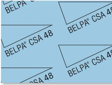
Compressed sheets for gasket made of mineral fibre, aramide and dispersed inorganic loads mixed in a matrix of type NBR rubber. The material is a sheet for gaskets for a wide range of applications. Its high compressibility, chemical resistance and good permeability make the BELPA CSA-48 suitable for most common uses, (water, air, oils, solvents, etc). It is also available with steel wire reinforcement and anti-stick coating. REF. BELPA CSA-48 M.
